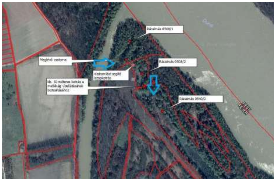
Map no. 1: Opening of the sidearm (the inflow section is shown by blue arrows) by dredging the previously used old inflow channel. With this action a steady and slow supply of water is expected, which would help preventing the future deposit of sludge.
